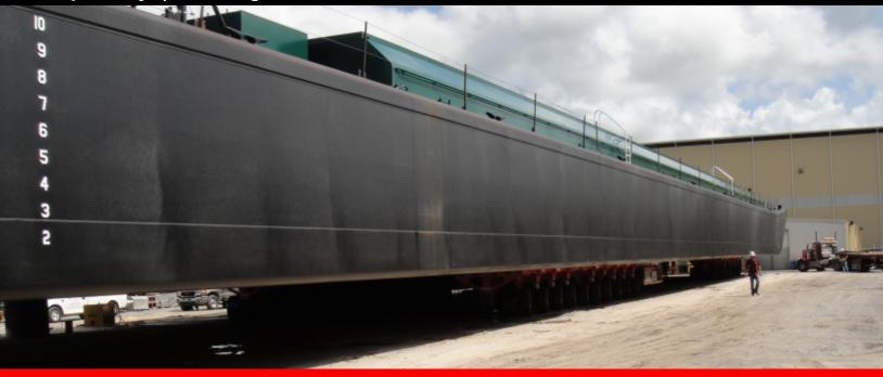
It was just another day on the job for the Berard Team loading out this 515 ton, 222'long x 54' wide barge. The vessel was loaded onto the customers launch barge system using twenty-four lines of ESE's and four power pack units. The team worked hand in hand together with the customer's employees to make the move a safe one, resulting in a job well done and a happy customer.
